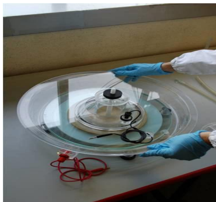
Figure 2: The assembled chamber to perform P-Dimensional electrophoresis.
