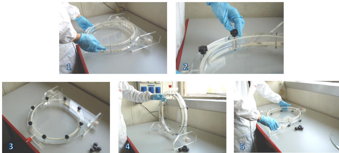
Figure 6: 1) Place the caster in horizontal position, with the front panel facing down; 2-3) fix the backside panel using the thumbscrews, 4-5) rotate the caster and place it in horizontal position with the backside panel facing down.
